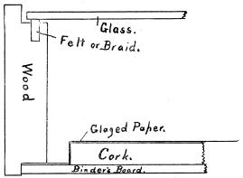
The boxes used for the collection are made as shown in the accompanying figure, and are from their peculiar construction not liable to warp or crack, and so remain perfectly insect-proof.
