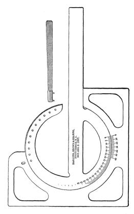
ment, which give the settings that are necessary. In many instances the protractor takes the place of the ordinary 45-degree and 60-degree triangles, and it is also used as an extension to the T-square when the work is beyond the end of the blade of the square. It is made by Darling, Brown, and Sharpe, manufacturers of fine tools, of Providence, R.I.
