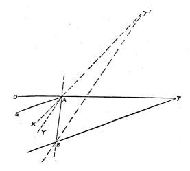
scale will indicate the distance AT'; but this reading will by no means be the same as that obtained when the object was at T, because the angle XAY is smaller than DAE. In other words, it is impossible to construct a scale giving true distances of objects from A in terms of the angle DAE, unless we impose as a condition that one of the sight lines shall make a fixed and constant angle with the base.
