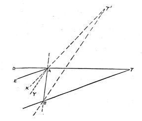
scale will indicate the distance AT'; but this reading will by no means be the same as that obtained when the object was at T, because the angle XAY is smaller than DAE. In other words, it is impossible to construct a scale giving true distances of objects from A in terms of the angle DAE, unless we impose as a condition that one of the sight lines shall make a fixed and constant angle with the base.
