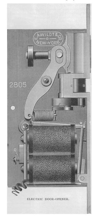
per left-hand corner of the electro-magnet, against which the latchbolt lever bears. The action of the opener is as follows: When the circuit is closed by a touch on the button, the armature is attracted by the electro-magnet; the tongue moves, thereby releasing the spiral spring, which pulls back the latch-bolt; and at the same time the coiled spring forces the door open by means of the throw back.
