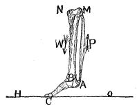
crum, but just there is the question. Suppose a person sitting down to put his toe against some object, and, by the same muscular action which raises the body on tiptoe, to push the object away. Here the case is evidently a lever of the first class, the ful-
