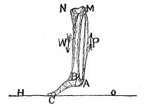
crum, but just there is the question. Suppose a person sitting down to put his toe against some object, and, by the same muscular action which raises the body on tiptoe, to push the object away. Here the case is evidently a lever of the first class, the fulcrum being the ankle-joint (B), and the weight the point of the toe's pressure (C).
