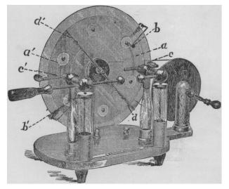
negative from the comb c, and leave the discharging-rod connected with it charged with positive electricity.
