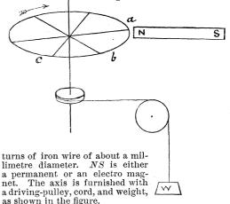
That part of the ring which lies between a and c is heated to bright redness by means of two or three Bunsen burners. The magnet then exerts a preponderating attraction upon the farther or cool side of the ring, and the latter revolves as indicated by the arrow. As fast as the ring enters the space a b c, it becomes red-hot and non-magnetic, and a lack of equilibrium is thus maintained which results in a continuous rotation.
