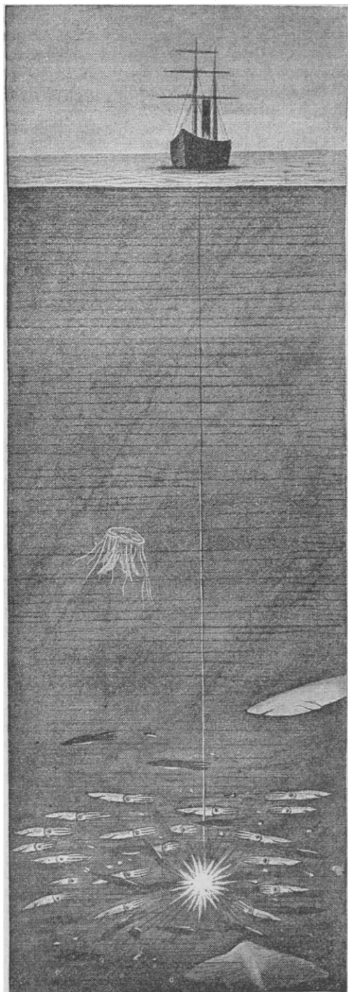
FISH-COMMISSION STEAMER ALBATROSS. A SUBMERGED ELECTRIC LIGHT TO ATTRACT FISH, AND ILLUMINATE THE WATER.
