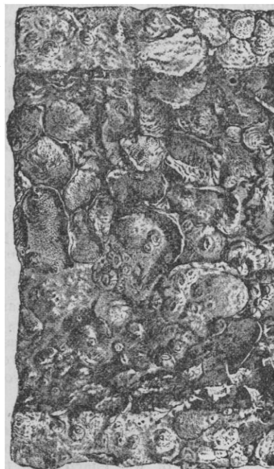
FIG. 2.—LOWER SIDE OF TILE EXPOSED JULY 9-AUG. 23. (TWO-THIRDS NATURAL SIZE.)
