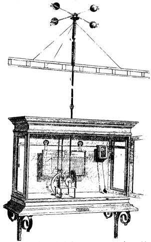
The four hemispherical cups, a a a a, turned round by the wind, impart their motion to a vertical shaft, b b, at the bottom of which is the endless screw, c, its lower end resting in a small agate cup filled with oil, connected with the train of wheelwork turning the cam, dd. At e, is the pencil resting on the edge of the cam; ff is a sheet of ruled paper attached to the board, gg, by means of small brass clamps, which is drawn aside at the above mentioned rate by the clock, k.
