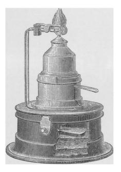
The pile is an element to the bichromate of potash, in which the liquid is replaced by a kind of amianthus saturated with a bichromatic solution similar to that of the pile jar.
