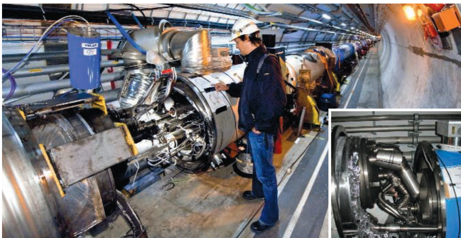
Blasted! A pressure wave within the LHC shoved 35-metric-ton magnets off their supports and mangled the connections between them.
