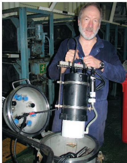
On board. FerryBox advocate David Hydes works with a ship-based sensor of CO 2 in water.
