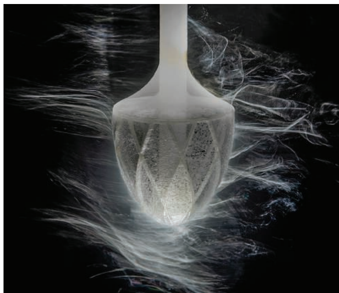
Microfibers are precisely deposited onto a rotating heart ventricle mold by using focused rotary jet spinning.
