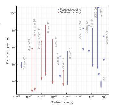
(10), which demonstrated cavity cooling of an electromagnetically trapped nanoparticle to its ground state]. Our result ("aLIGO") sets a new record in the macroscopic mass range, reaching 10.8  $\pm$  0.8 phonons. Experiments with future gravitational-wave interferometers ("3G") will achieve occupations <1.
