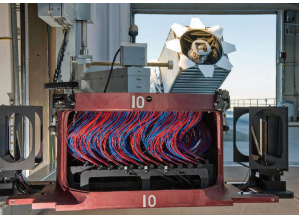
Hundreds of fibers, arranged by hand, capture light at the Sloan Digital Sky Survey's New Mexico telescope.
