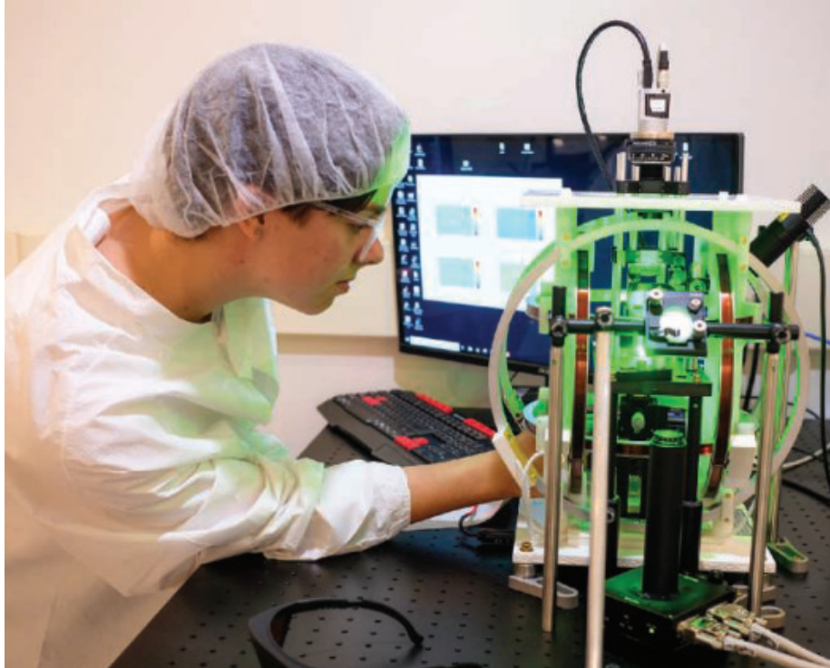
A quantum diamond microscope contains a doped diamond slide that is excited by tiny magnetic fields.
