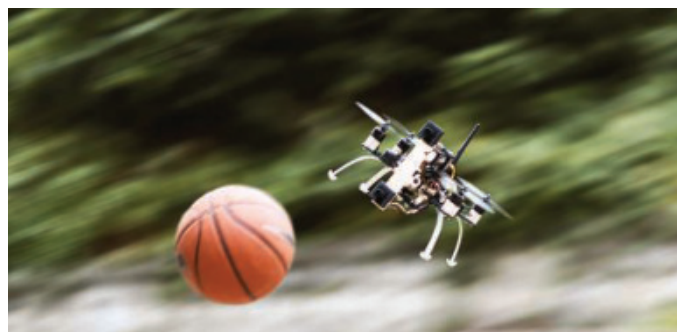
A drone dodges objects using event-based cameras and onboard processing.
