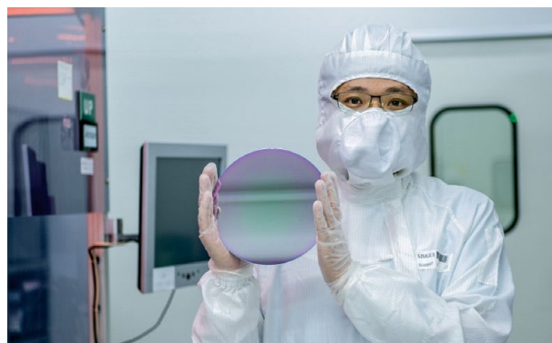
The first independently developed 8-in. radiation-hardened silicon-on-insulator (SOI) wafer, manufactured by SIMIT
