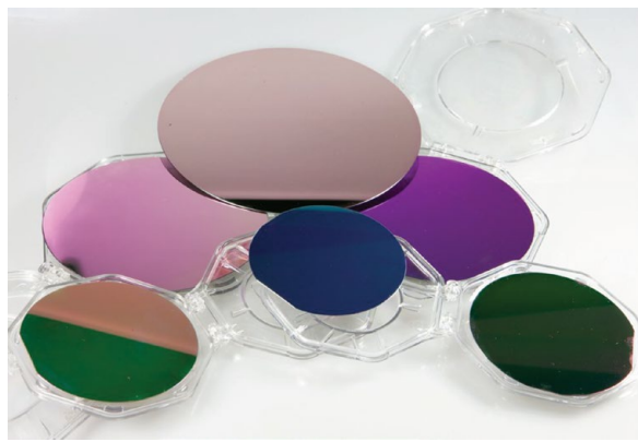
Examples of silicon-on-insulator (SOI) wafers fabricated by SIMIT
