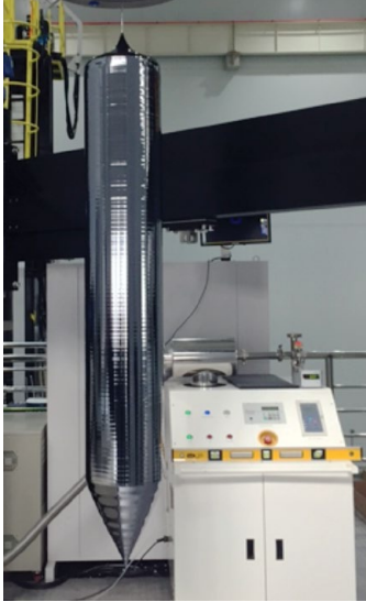
Shanghai Zing Semiconductor Technology Co., Ltd., successfully produced the first 300-mm single-crystal ingot in China.
