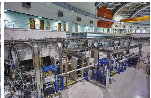
SiP.ME 2 beam lines and stations for in situ characterization of the electronic structure of energy and environmental materials
