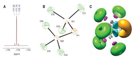
Fig. 3. Characterization of phosphide 1. (A) <sup>31</sup>P NMR spectrum of [TBA][1] displaying <sup>29</sup>Si satellites.
