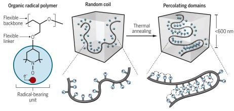
Pendant radical groups on the polymer backbone bear highly localized electrons. Unannealed, these radical groups are too far apart to transport electrons over large distances. Annealed, the radical groups organize into percolating domains that facilitate electron transport.
