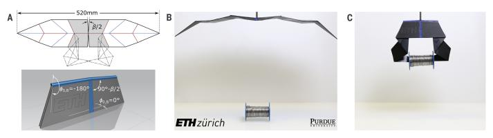
Fig. 5. Spring origami gripper (movie S2). (A) Fold pattern. Gray facets and computer-assisted design model: preprogrammed control cell. White facets:
