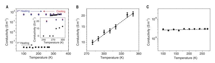
**Fig. 3. PTEO conducts charge after annealing has occurred.** (**A**) Electrical conductivity as a function of temperature for PTEO in a 0.5-µm channel. Real-time annealing of the thin film allowed for local order to appear within the film so that the electrical conductivity was altered by 10 decades. (**B**) Above the glass transition temperature, there is thermally
