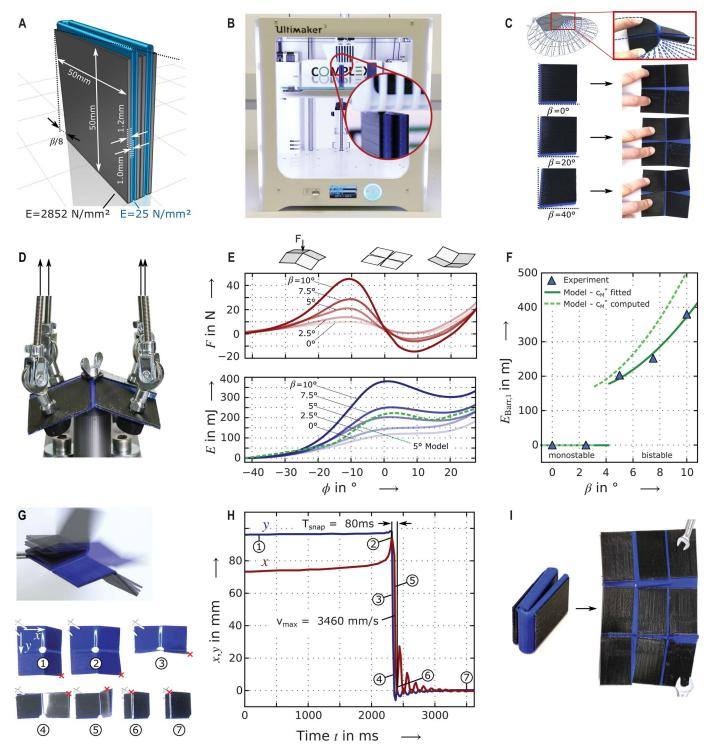
Fig. 4. Four-dimensional printing and experimental investigation of spring origami mechanisms. (A) Geometry and material properties.
