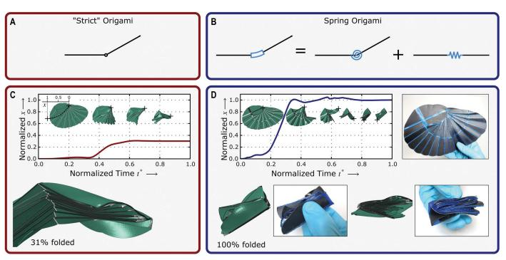
Fig. 2. Assumptions and FEA simulations describing the self-folding behavior of the earwig wing. (A) Strict (rigid) origami model.
