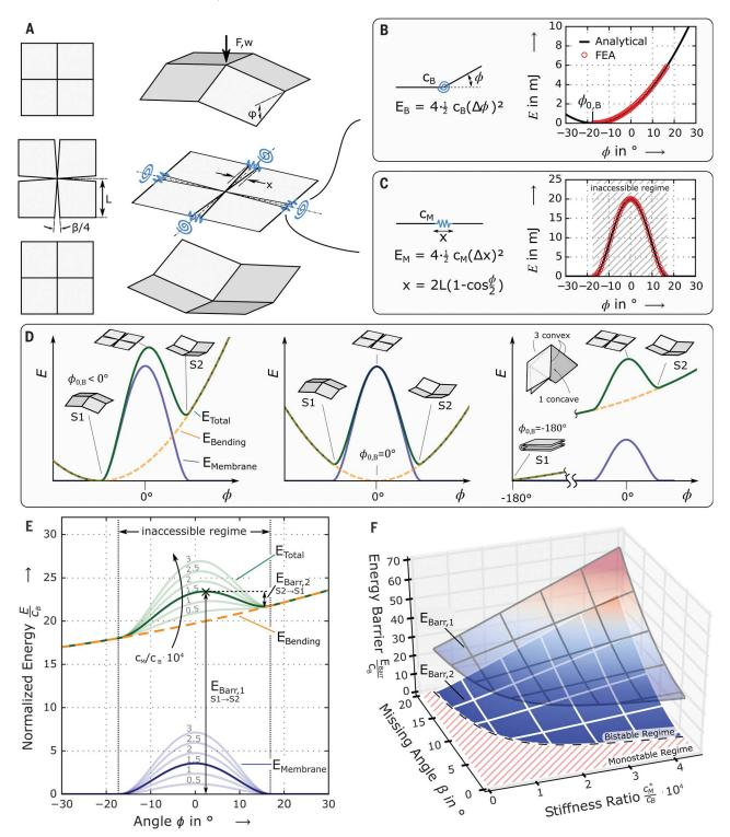
Fig. 3. Generalized model of bistable four-fold spring origami
