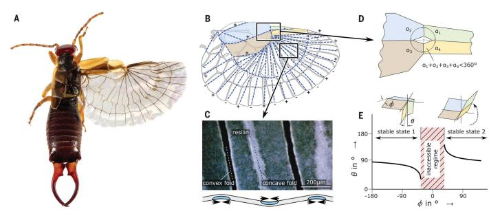
**Fig. 1. Earwig wing as a natural example of multifunctional programmable folding. (A)** The earwig *Forficula auricularia* with unfolded wing. [Image reprinted with permission from G. Wizen] (**B**) The folding pattern is incompatible with rigid origami assumptions. [Image adapted from Haas *et al.* (19)] (**C**) Alternating, asymmetric resilin distribution throughout the wing drives the self-folding process. The schematic under the
