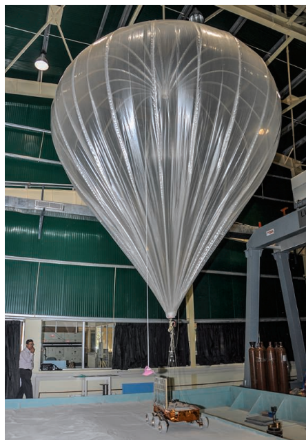
To simulate the moon's anemic gravity during testing of its lunar rover, the Indian Space Research Organisation tethered a model to a helium balloon.
