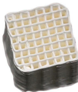
A printed cubic lattice scaffold for the creation of porous ceramics
