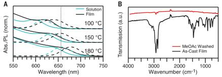
**Fig. 3. CsPbl<sub>3</sub> QD films. (A)** UV-visible absorption (solid lines) and PL spectra (dashed lines) of CsPbl<sub>3</sub> QDs in solution (blue) and as-cast films (black) for QDs synthesized at 100°, 150°, and 180°C. (**B**) FTIR spectra showing the IR transmission of a CsPbl<sub>3</sub> QD film as cast (black) and after treating with MeOAc (red).
