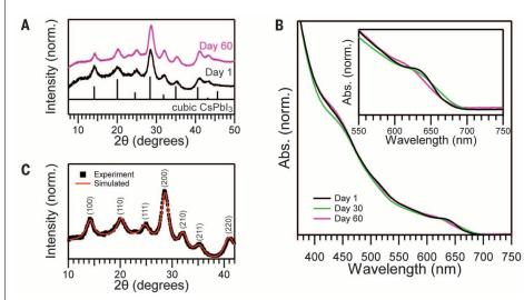
**Fig. 2. Phase stability of CsPbl<sub>3</sub> QDs. (A)** Powder XRD patterns and **(B)** UV-visible absorption spectra, normalized at 370 nm, of CsPbl<sub>3</sub> QDs synthesized at 170°C and stored in ambient conditions for a period of 60 days. (Inset) The slight blue shift that is seen in the excitonic peak with extended storage. **(C)** Rietveld refinement fitting of CsPbl<sub>3</sub> QD XRD pattern, revealing pure cubic-phase CsPbl<sub>3</sub>.
