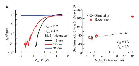
**Fig. 4. MoS**<sub>2</sub> **thickness dependence.** (**A**) Dependence of MoS<sub>2</sub> channel thickness on the performance of 1D2D-FET. SS increases with increasing MoS<sub>2</sub> channel thickness. (**B**) Extracted SS from experimental curves and TCAD simulations show increasing SS as channel thickness  $T_{CH}$  increases.
