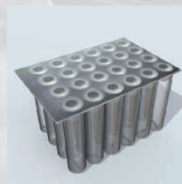
Four sets of preweighed catalysts in glass microvials with stir bars.
