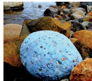
"Smart rock" with an embedded accelerometer and radio frequency identification tag
