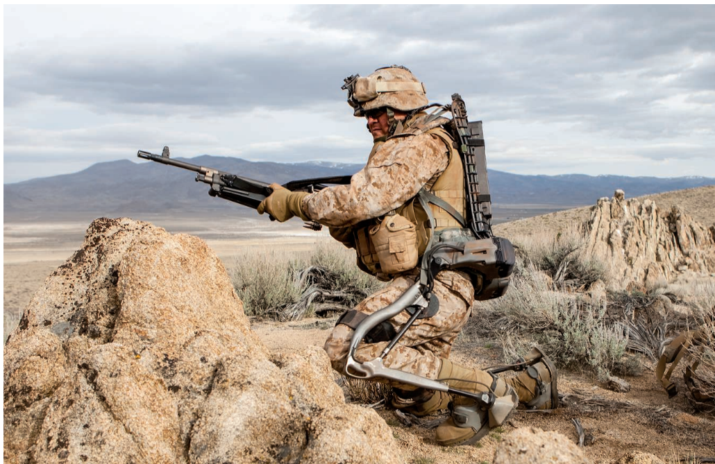
The HULC, a rigid, battery-powered exoskeleton developed by the U.S. military in the late 2000s, failed to deliver predicted performance boosts. Wearing the suit "was a workout," one tester said.
