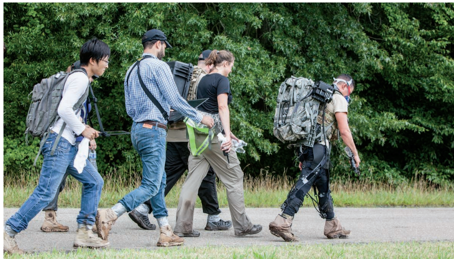
A team of technicians trails a military exosuit tester, gathering data that will reveal whether the device is aiding—or hurting—the soldier’s performance.
