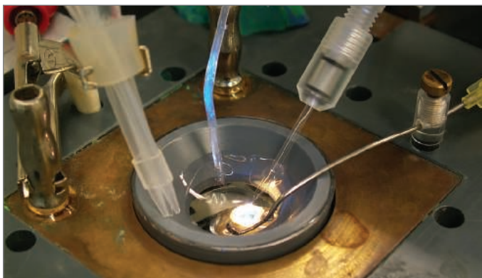
Patch clamping uses a tiny microcapillary tube to track fluctuations in a single neuron's ion channels.
