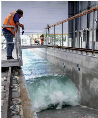
The new facility is 300 meters long and boasts waves as high as 4.5 meters.
