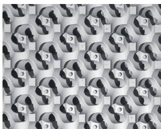
Surface of a 3D photonic crystal with four Weyl points in the band structure
