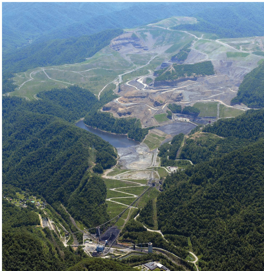
Scarred. Mountaintop mines, such as this one in West Virginia, end up filling stream valleys with tons of debris, creating wedges of rubble (center). The waste leaches sulfate and other ions that harm aquatic life.
