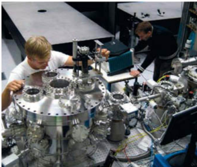
Looking in. In the Garching experiments, atoms in the cylindrical chamber were blasted with attosecond pulses and laser waves.
