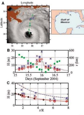
measured  $H_{\rm s}$  reached 17.9 m at a radial distance of 73 km, about 30 km from the strongest winds. Furthermore, our measurements, from the forward face of Ivan, are likely ~85% of the maximum  $H_{\rm s}$  typically found in the right quadrant (4, 6). These factors strongly suggest the wave field associated with Ivan should generate maximum  $H_{\rm s}$  values greater than 21 m and  $H_{\rm max}$ values greater than 40 m at r/R = 1.
