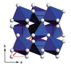
**Fig. 4.** Crystal structure of pyrite-type silica. Coordination polyhedra of O atoms around Si atoms are shown as octahedra. O atoms are illustrated as balls. The black line indicates the unit cell, and bold red lines show the second nearest bonds. 6+2 coordination polyhedra are illustrated by dotted red lines.
