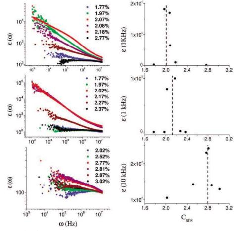
**Fig. 1. (Left)** Dielectric constant of nanotube dispersions versus frequency for different micelle weight fractions, indicated by different colors. The nanotube volume fractions are, from top to bottom, 0.19, 0.13, and 0.06%. (**Right**) A determination of the surfactant concentration corresponding to the percolation threshold by identifying the points where the dielectric constant at low frequency is maximum. The percolation is indicated by the dashed lines.
