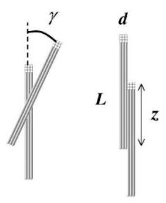
Fig. 3. Schematic of interacting nanotube bundles. (Left) The bundles are in contact at an angle  $\gamma$ . (Right) The bundles are in contact and parallel. *L* and *d* are the length and the width of the bundles.
