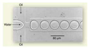
**Tunable droplets.** Water droplets form at a rate of 1000 per second in an asymmetric microchannel containing hexadecane. The channel is  $30 \,\mu$ m high.
