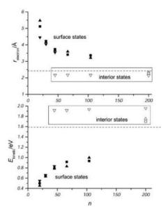
**Fig. 4.** Radius of gyration and kinetic energy of the excess electron in water-cluster anions at three simulation temperatures, 100 K ( $\nabla$ ), 200 K ( $\Delta$ ), and 300 K ( $\square$ ). Filled symbols denote surface states, open symbols denote interior states. The dashed lines show the simulated radius of gyration and kinetic energy of the hydrated electron in bulk water at 298 K (*10*). The surface-state data behave comparably to the experimental data [see figure 1 in (*19*)].
