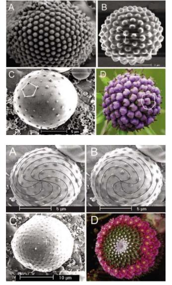
core/shell of ~9.5  $\mu$ m in lateral dimension (Fig. 2, A and B), the 92 spherules can be assigned to eight clockwise and five counterclockwise spirals, and thus they form a 5 by 8 Fibonacci number pattern. In Fig. 2C, the lateral dimension for the core/shell is about 18  $\mu$ m, and the spherules, about 230 in total, form a 13 by 21 Fibonacci number pattern, similar to the one on the cactus *Mammillaria nejapensis* (Fig. 2D).
