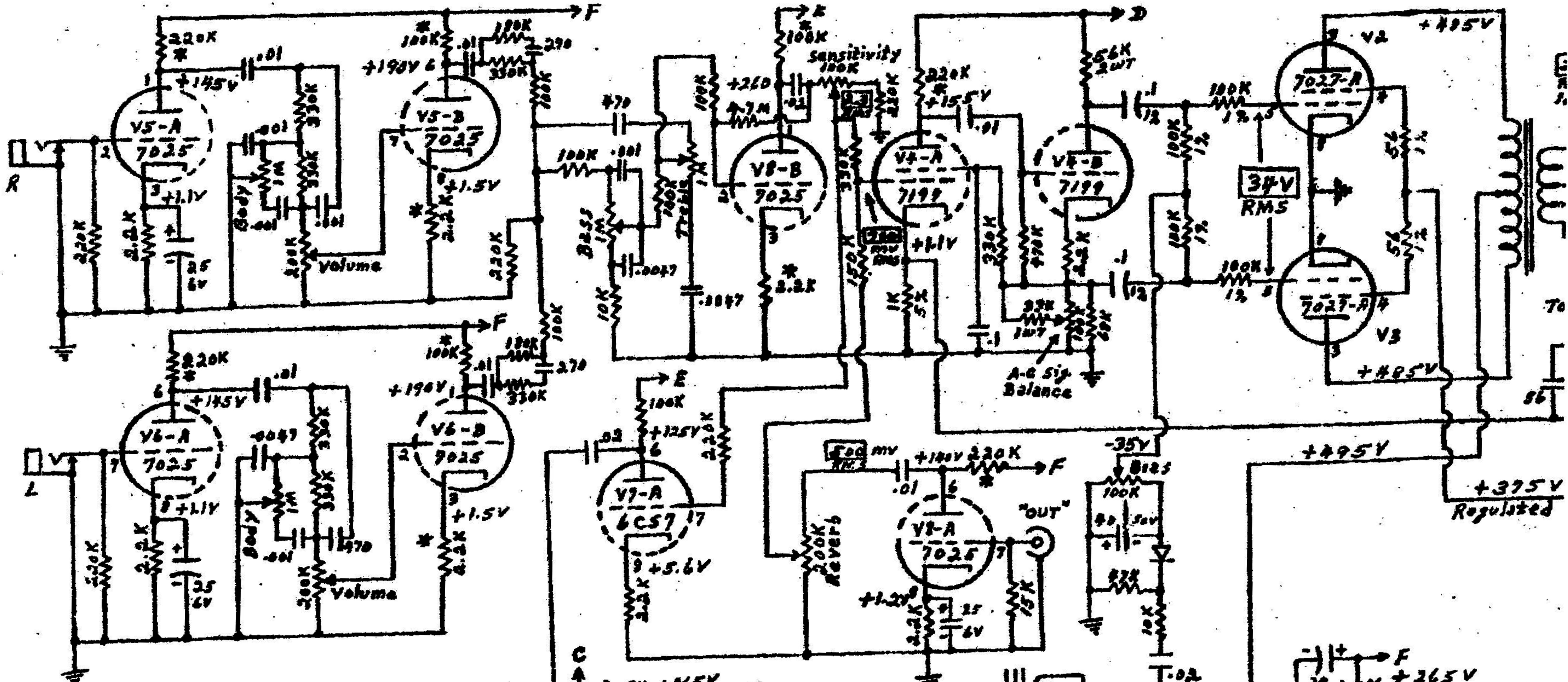
1. \* Indicates low-noise film resistor, 1-w.
