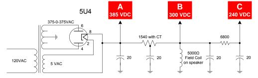
This simplified schematic is electrically correct, but has purposefully omitted interconnection plugs and jacks to make the schematic easier to understand. The AC primary circuit, fuses, switches, relays, etc. have been omitted for the same reason.
