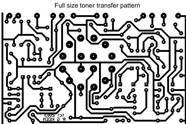
The full sized PCB layout is shown at bottom left, and the parts stuffing diagram and wiring diagram is at left. Pots are show viewed from the back.
