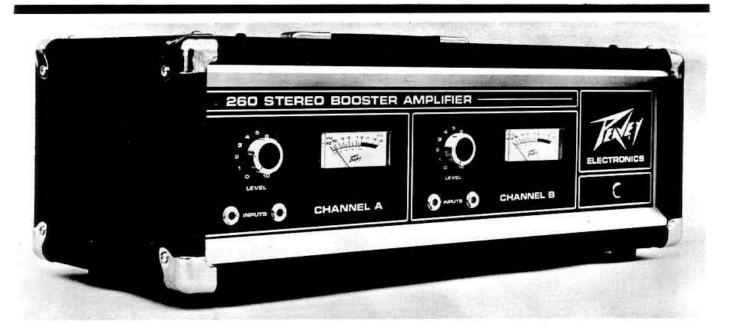
The new 260 Stereo Booster uses four high voltage 30 amp power devices in each channel to deliver 130 watts RMS per channel, both channels driven simultaneously into 4 ohms, with a frequency response of 20 Hz to 20 kHz. One channel can deliver as much as 140 watts RMS. The output devices are mounted on a massive aluminum heatsink for continuous duty. Additional ther-
