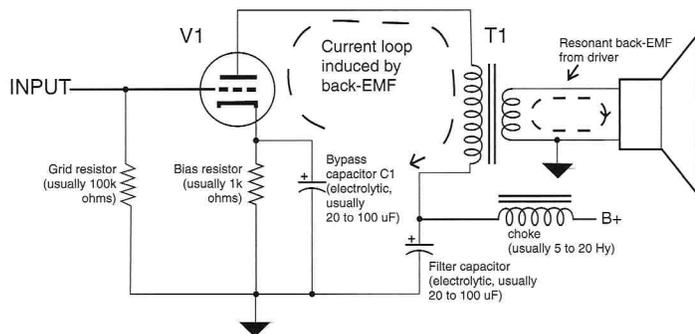
**Figure 3: Path of back-EMF through SE triode amplifier.**
