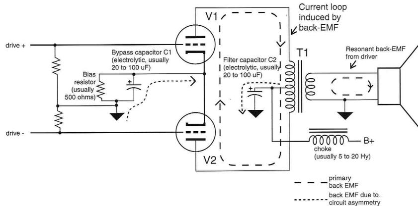
**Figure 4: Path of back-EMF in push-pull triode amplifier.**
