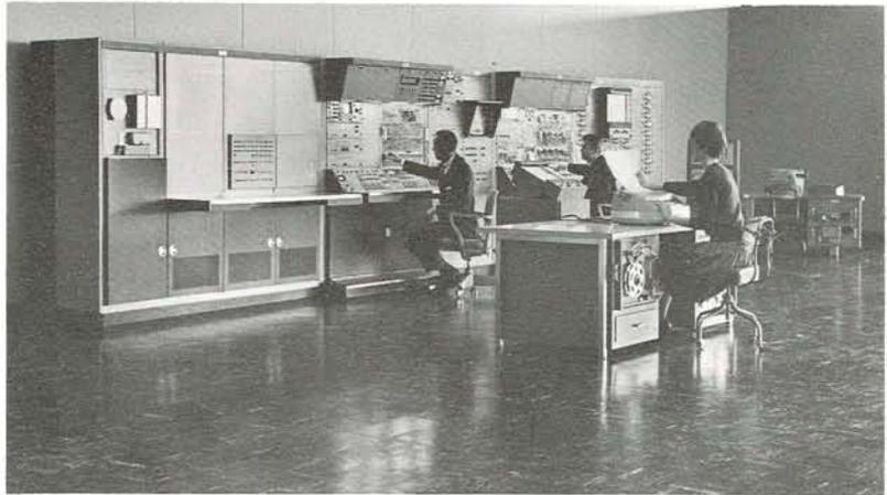
EAI HYDAC 2400 — a powerful new tool for scientific computation . . . a completely integrated hybrid computing system to provide solutions to problems beyond the scope of separately operated analog or digital computers.
