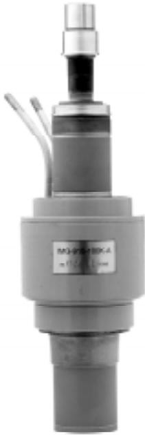
**T**he ISTOK™ IMG-915-100KA Industrial Magnetron is a 915 MHz fixed-tuned, electromagnet-focused 100 kW CW magnetron. It features ceramic-metal construction, liquid and air cooling, and very rugged construction for industrial applications.
