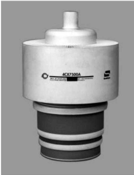
**T**he Svetlana™ 4CX7500A is designed for audio and radio frequency applications. The Svetlana 4CX7500A has a directly-heated thoriated tungsten mesh filament for mechanical ruggedness, good VHF electrical performance and high RF efficiency.
