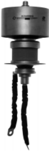
**T**he Svetlana™ 3CX6000H3 is a highly reliable ceramic/metal power triode designed for use in amplifier or oscillator service. A modern mesh filament is used, ensuring better mechanical rigidity and long lasting concentricity of the filament, contributing to longer life. Flexible leads connect to the filament terminals and a mounting flange provides the grid connection. The flange provides a convenient way to mount the tube.
