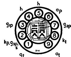
The BRIMAR ECL82 and PCL82 are noval triode-pentodes for use in frame time-base circuits and as sound amplifiers and output valves.
