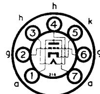
The BRIMAR 6AF4A is intended for use as a U.H.F. oscillator valve up to 1000 Mc/s.
