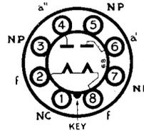
The BRIMAR type 5U4G is a full-wave directly heated rectifier for use in A.C. equipments which require more power than type 5V4G will provide.
