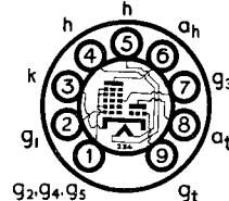
The BRIMAR 20D4 is a triode-heptode frequency changer on the Naval (B9A) base, featuring very high conversion conductance.
