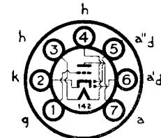
The BRIMAR 12AE6 is a double diode triode for use in detector, A.V.C. and A.F. amplifier circuits of car radio receivers and is intended to operate directly from the 12-volt battery without the use of a vibrator H.T. system. It is designed to operate over the range of voltage variations normally encountered with car batteries.
