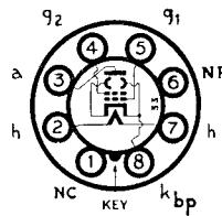
The BRIMAR type 12A6 is an indirectly heated output beam tetrode of high efficiency for use in car radio or A.C./D.C. receivers, where the supply exceeds 110 volts.
