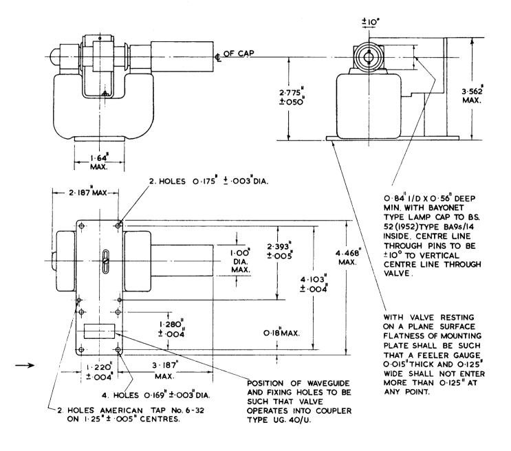
**General.** The M 503 is an air-cooled multi-resonator packaged magnetron, with a pre-plumbed waveguide output circuit. It has been designed for operation in the 3 cm band and is for use with systems using the standard American waveguide; the internal dimensions of which are  $0.9 \times 0.4$  in.
