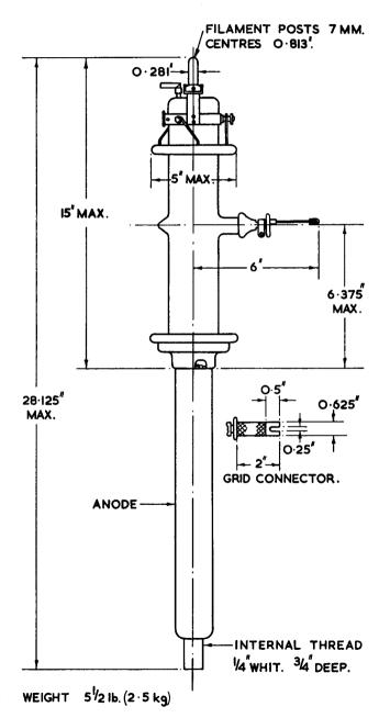
for at least 1 hour at half the normal anode voltage and current. The anode voltage should then be increased slowly to the normal value. During this process a resistance of at least 25  $\Omega$  should be connected into the anode supply lead, in order to limit the surge current in the event of a flashover inside the valve.
