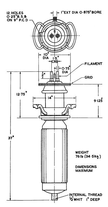
Mounting. The valve must be completely supported by its water jacket, which should be adjustable so that the axis of the valve may be made truly vertical. Rigid connection must be made to the anode only.
