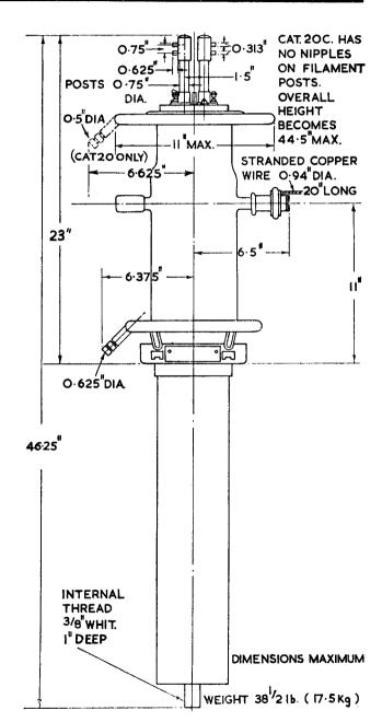
Mounting. The valve must be completely supported by its water jacket, which should be capable of adjustment so that the axis of the valve is truly vertical. Rigid connections must be made to anode only.
